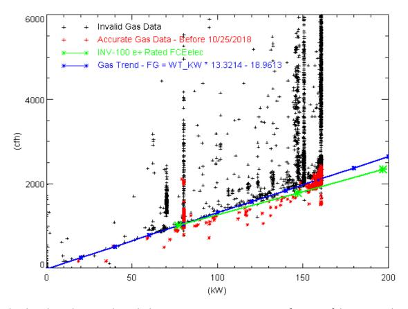
The developed trend was used to calculate system gas consumption as a function of the measured gross power output.
